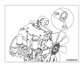
(7) Operate the engine at low idle and inspect for leaks at the filters and the drain plug. Shut the engine off and check the oil level with the dipstick. Allow 15minutes for oil to drain down before checking.
