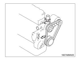
(2) Inspect the drive for damage.
