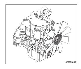
(4) Apply a light film of lubricating oil to the gasket sealing surface before installing the filters.
