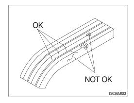
(3) Inspect the drive belt, tension bearing and fan hub.
