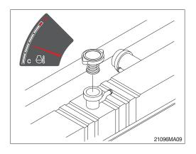
▲ Wait until the temperature is below 50°C (122°F) before removing the coolant system pressure cap.
